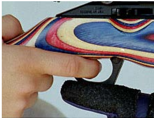
Take up the slack (first-stage) on the trigger and then, with the sights aligned on the target, smoothly press the trigger to the rear until the mechanism releases.
