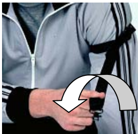
4-a. Extend the sling and rotate the sling swivel one-half turn to the right (clockwise direction).
